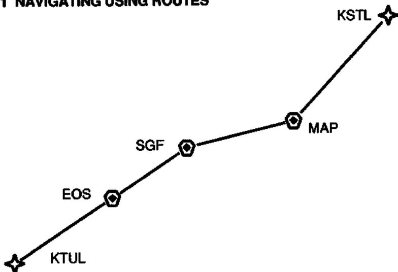
Route 0 is called the active route and is the route used for navigation. The waypoint toward which you are navigating is called the “active to” waypoint. The waypoint immediately behind you is called the “active from” waypoint. The line defined by two consecutive waypoints in a route is called a “leg”. For example, the waypoints EOS and SGF form a leg. The leg that connects the “active from” and “active to” waypoints is called the “active leg”.
