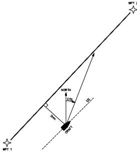
As an example, suppose you activate the route illustrated above. The GPS 100 chooses the closest leg with a desired track of 45 degrees but your position happens to be 2 nautical miles off course. The unit will automatically compute the optimal course to steer (which is 15° in this example). Simply go to the CDI page, select “CTS” on line 2, and “TRK” on line 3. Turn your craft such that your track (TRK) matches the recommended course to steer.
