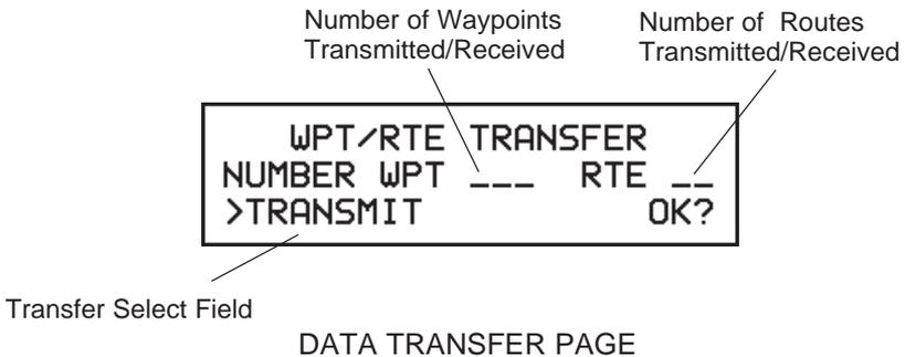
Waypoints and routes may be transferred from one GPS 100 to another, or from a PC to a GPS 100. The Data Transfer Page allows you to select the desired data transfer operation (receive waypoints/routes or transmit waypoints/routes). Data transfer operations require an optional PC kit or data transfer cable.
