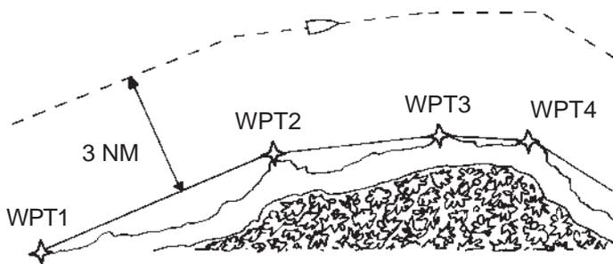
Parallel offset navigation, introduced in Section 11.4, can be extremely useful in either the marine or aviation environment. Offset navigation allows you to translate your course to the left or right of the actual route by a distance you choose. This feature can help you stay clear of dangerous areas and can also help with specialized navigation such as shrimping, weather avoidance, airway navigation, or search and rescue.
