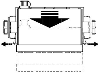
**To remove the GPS 100 from the slide mount...**
