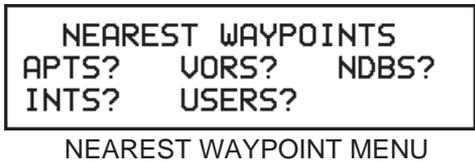
An important feature of the GPS 100 is the ability to display waypoints nearest to your position. In an emergency, you may use the nearest waypoint feature to find the closest point of safety in your area. Up to 9 waypoints, closer than 200 nm, are computed for each type of waypoint. To view a specific waypoint type, place the cursor over the desired type and press the ENT key.
