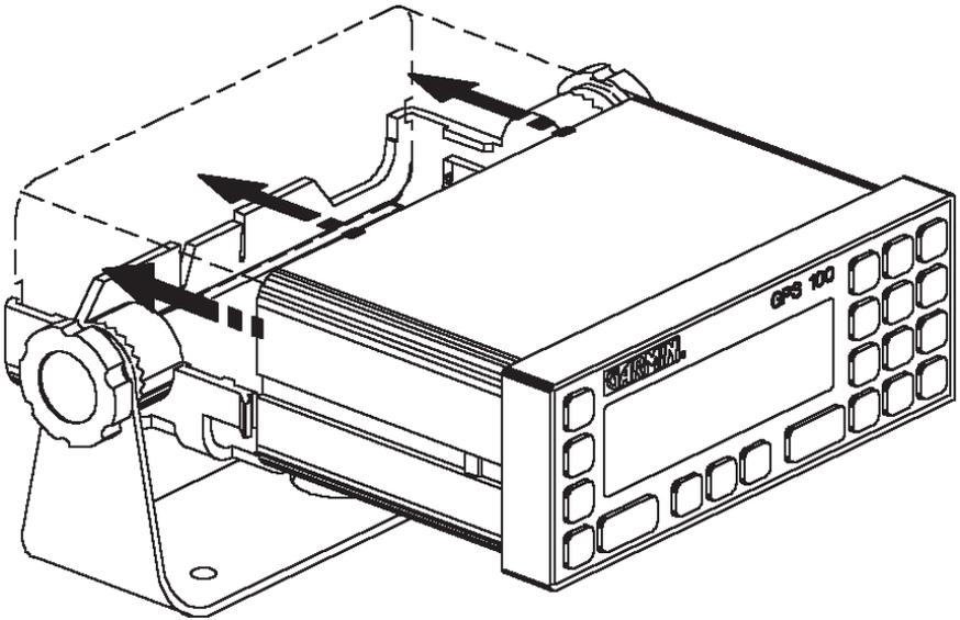
**To insert the GPS 100 into the slide mount...**
