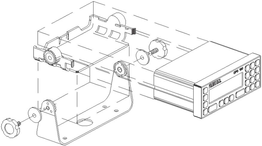
The GPS 100 comes with a standard slide-in gimbal bracket for fixed installations. The gimbal bracket may be mounted on a flat surface or overhead using screws or bolts.
